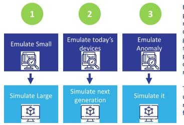
Emulation and simulation tools (Figure 2) are part of SCP. These tools can model large-scale networks that are not practical to build until deployment. They also help simulate nextgeneration devices for features such as links speed and capacities not yet available and provide the engineer with unparalleled observability of the root causes of production network performance anomalies.
